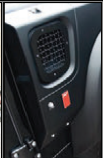
Side Vents with Mesh Stainless Steel - Supplied Powder Coated in Black
