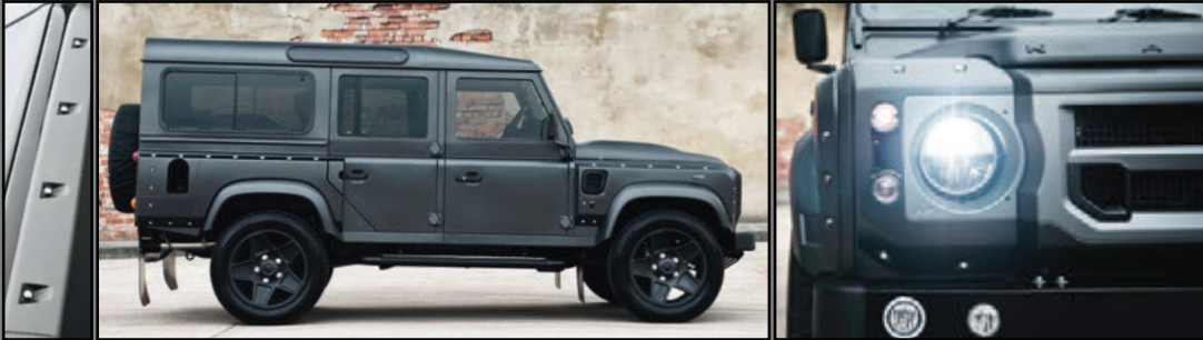
Defender 110 - Front & Rear Wider Wings with Integrated Vents & Bolt Apertures Carbon Composite 07 X - Lander Front Grille With Headlamp Surrounds 10
