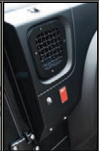
Side Vents with Mesh Stainless Steel - Supplied Powder Coated in Black
